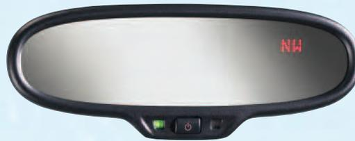
This small, oval-shaped auto-dimming mirror supports the Audi TT's styling and comes with a red transreflective compass display that matches the car's interior lighting scheme.
